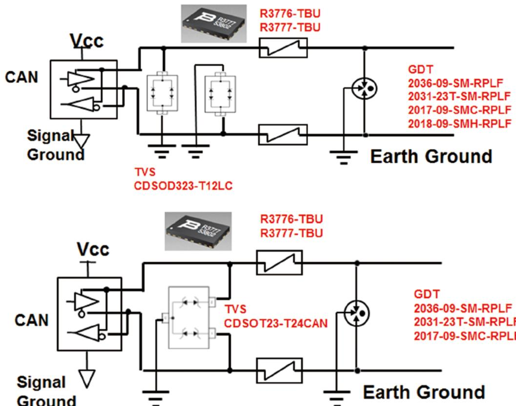
IEC61000-4-2 ESD (8kV/15kV) Level4, EMI
