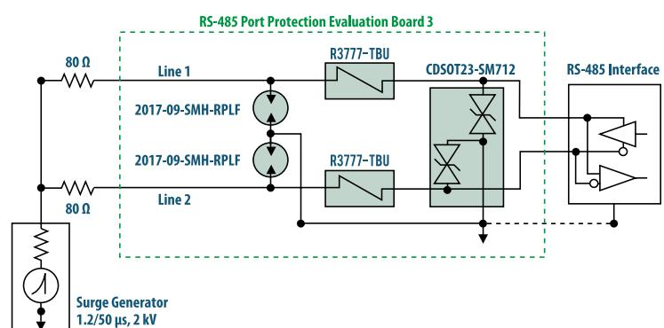
浪涌测试 2kV(1.2/50μs, Rext = 80 ohms)
