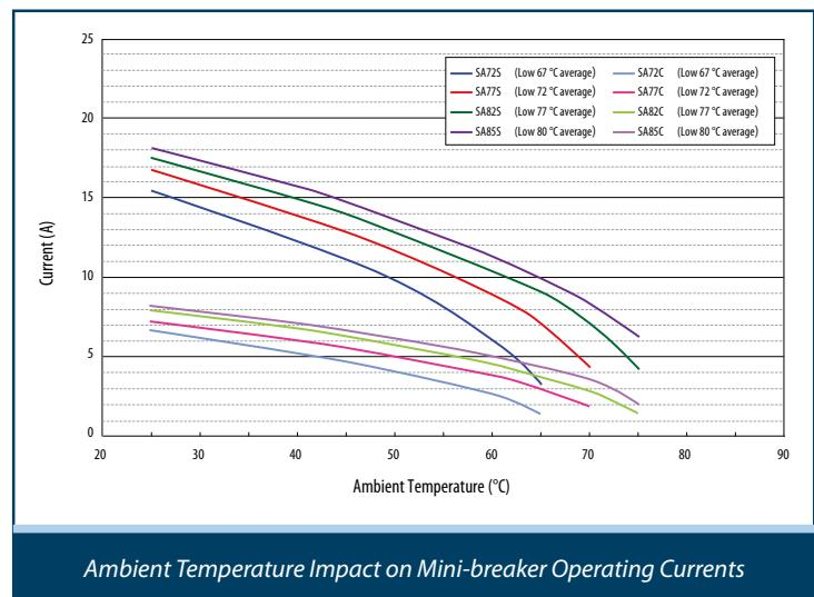
Ambient Temperature Impact on Mini-breaker Operating Currents
