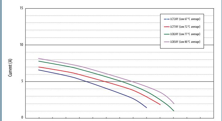
Ambient Temperature Impact on Mini-breaker Operating Currents
